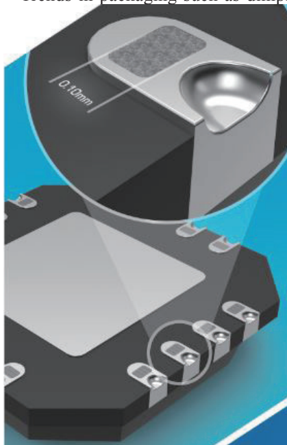
Figure 3: Wettable flank/dimple pad device.
